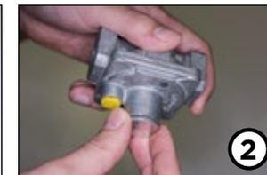
2 - UN SCREW THE CAP TO ACCESS THE REGULATOR ADJUSTMENT.
