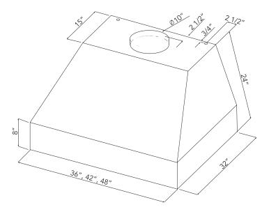
Made of the high quality 304 stainless steel, the Sedona Vent Hoods are engineered for beauty and performance. With simple design and elegant function, these vent hoods include 1200 cfm blowers, halogen lighting, and baffle filters for enhanced performance.
