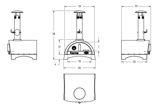
Figure X. Dimensions: 25in. Oven with Black, Powder Coated Cart
