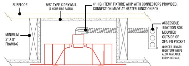
**STEP 3** Install the frame into the finished pocket. You may choose to leave all four inches of the trim exposed, or partially cover it with a decorative ceiling (1/2" clearance is required from ventilation holes).
