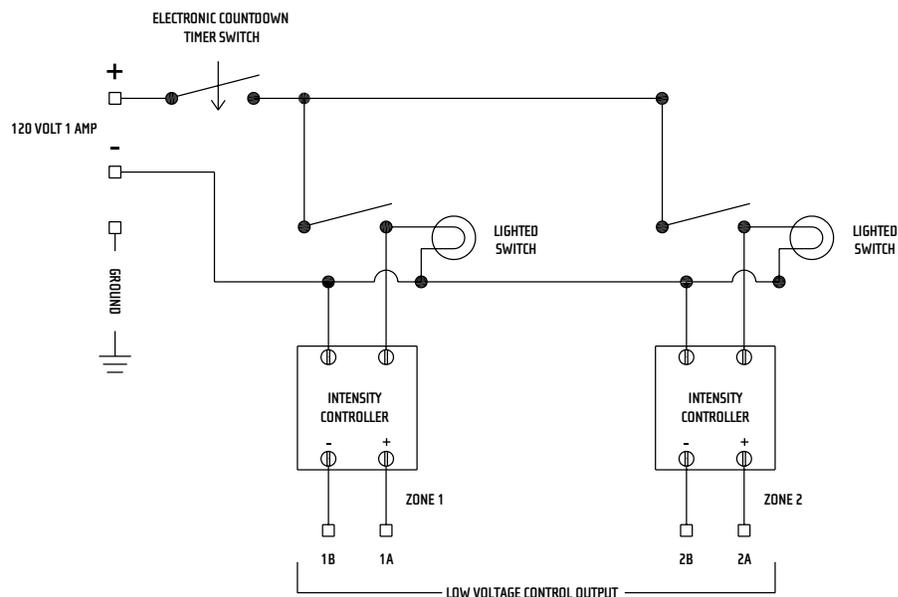
NOTE: USE TWISTED PAIR OR SHIELDED WIRE FOR LOW VOLTAGE HOOK-UP.
