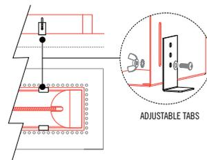
**WARNING: FRAME AND HEATERS CANNOT BE FLUSH MOUNTED ON A SLOPED/PITCHED CEILING. FLUSH MOUNT APPLICATIONS MUST ALWAYS BE INSTALLED WITH HEATERS HORIZONTAL TO THE FLOOR ON A FLAT, NON-SLOPED CEILING.**
