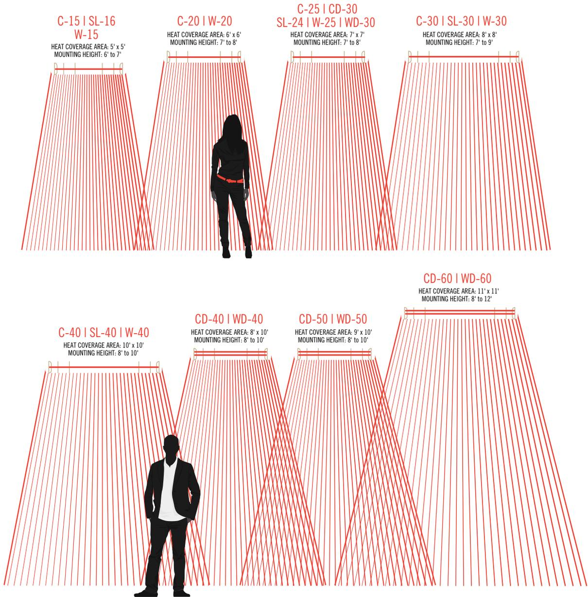
**NOTE:** Indoor or well-protected environments will generally exceed average coverage. Heaters may provide less than average coverage in extremely cold or windy conditions.
