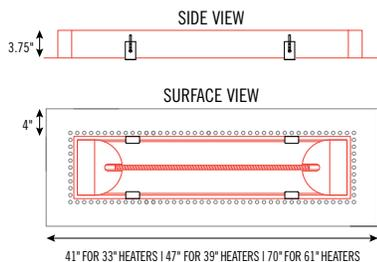
**STEP 4** Install the heater (heater must face horizontal to the floor) and adjust the tabs to set the heater flush with finished ceiling.
