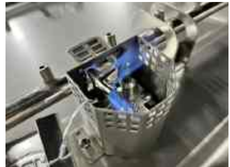
Figure 9.2 – Pilot flame coverage of thermocouple.
