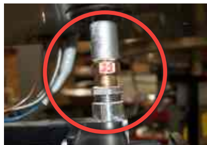
Figure 10.1 – Locating orifice for cleaning
