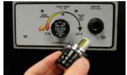
Figure 10.5 – Remove igniter unit cap with battery.
