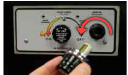
Figure 10.4 – Unscrew spark igniter unit cap.
