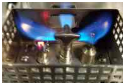
Figure 10.2 – Pilot flame coverage of thermocouple.
