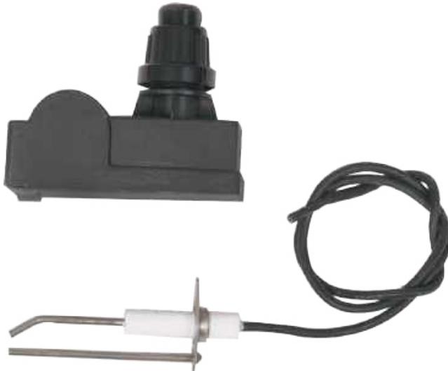
IK-1 UNIVERSAL SPARK GENERATOR PUSH BUTTON IGNITOR IGNITION NEEDLE WITH 22" L WIRE ONE OUTLET AAA BATTERY NOT INCLUDED 2 1/2" HIGH X 3" WIDE X 1 1/4" DEEP 3 OZ. MASTER PACK: 5 095192 199250
