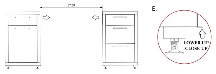
B. Place center panel between the drawer assemblies (it will rest on the inside bottom lip located on both drawer assemblies). You will need two people to align the drawer assemblies to the center panel. Once the center panel is in place and aligned the the front of the drawer assemblies use 6 screws to attach drawer assemblies to center back panel.
