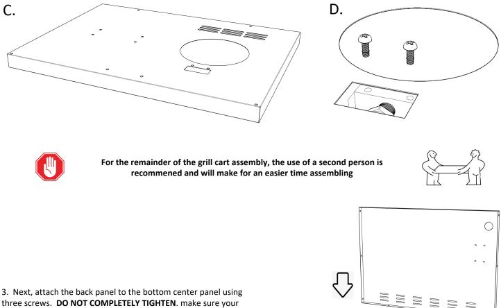
three screws. **DO NOT COMPLETELY TIGHTEN**. make sure your working on a soft surface to keep from damaging the product.
